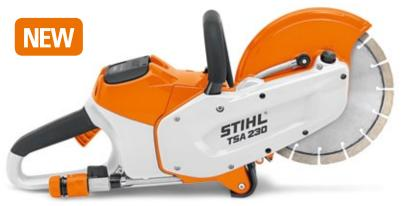
The world's first cordless cut-off machine with 230 mm cutting wheel for wet cutting. Suitable for indoor and outdoor use, up to 70 mm cutting depth, suitable for use in rain, water connection with ball valve and hose coupling, spindle lock, maintenance-free belt drive.
