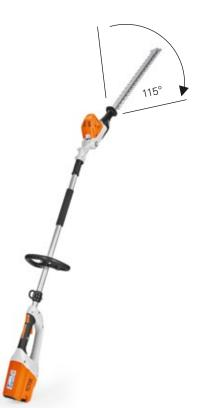
Cordless long-reach hedge trimmer for tall and wide hedges. Constant blade stroke regardless of the load, can be folded together, adjustable for vertical overhead and ground-level cutting, cutter bar adjustable by 115°, long reach, double-sided cutting blades, carrying length 125 cm, can also be used in the rain, total length 205 cm.
